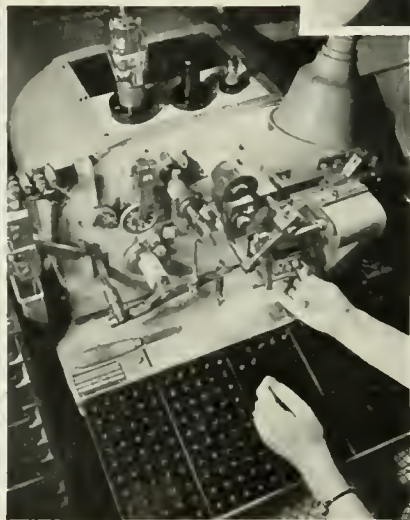
HAIR-LIKE TUNGSTEN WIRES ARE FOLDED INTO SHIPE ON THIS MACHINE.
